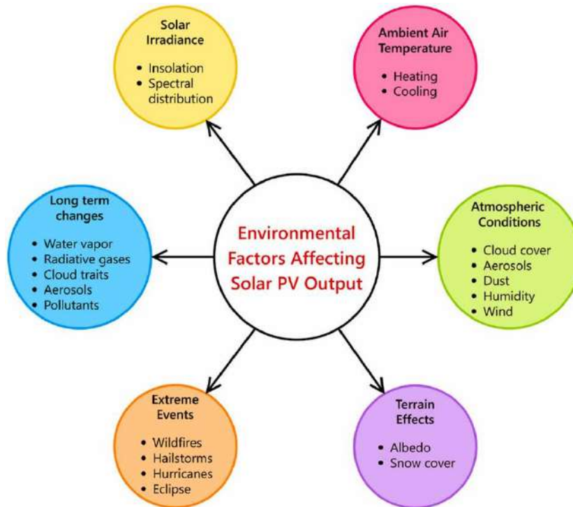
Figure 23: Environmental factors that affect Solar PV output (Bamisile et al., 2025)
